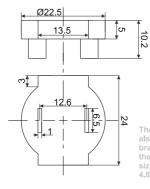
The B3P package also includes 2 brass terminals for the connector, the size of which is 4.8x0.5 millimeters
